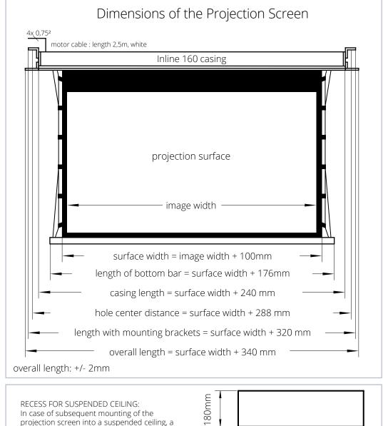
RECESS FOR SUSPENDED CEILING: In case of subsequent mounting of the projection screen into a suspended ceiling, a recess according to the sketch has to be made.
